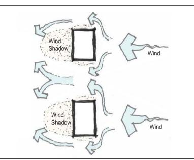
Diagram M: Plan showing how wind moves horizontally around buildings
